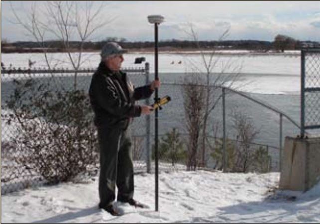
Des Rasch, OLS, owner of Rasch & Chambers Ltd. in Dunnville, Ontario, Canada determines a geodetic elevation point using the Can-Net GNSS Reference Station Network.
