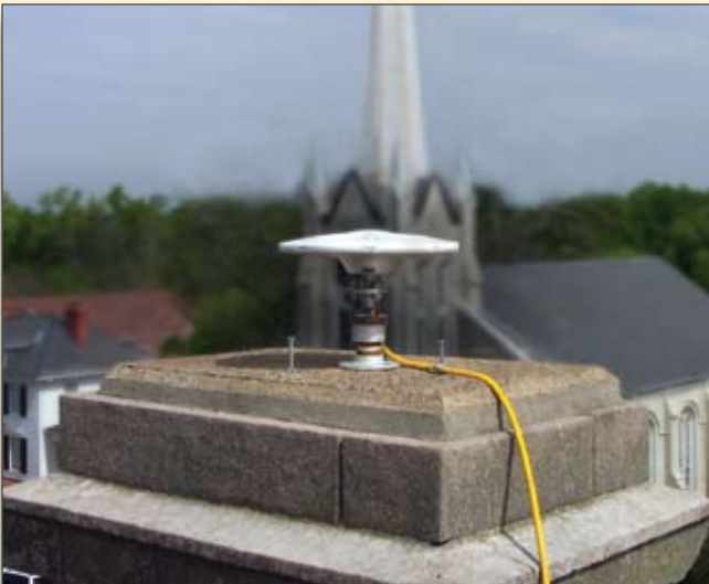
Trimble Zephyr Geodetic 2 antenna on top of South Carolina's York County Courthouse.
