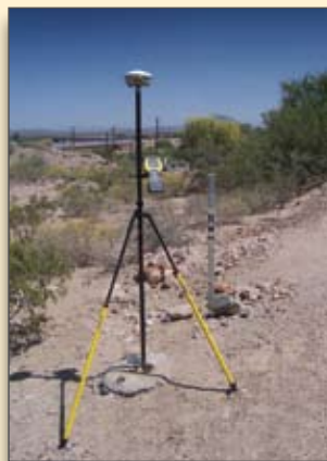
Trimble R8 GNSS rover checking NGS control point with the AZGPS GNSS network in Phoenix, Arizona.
